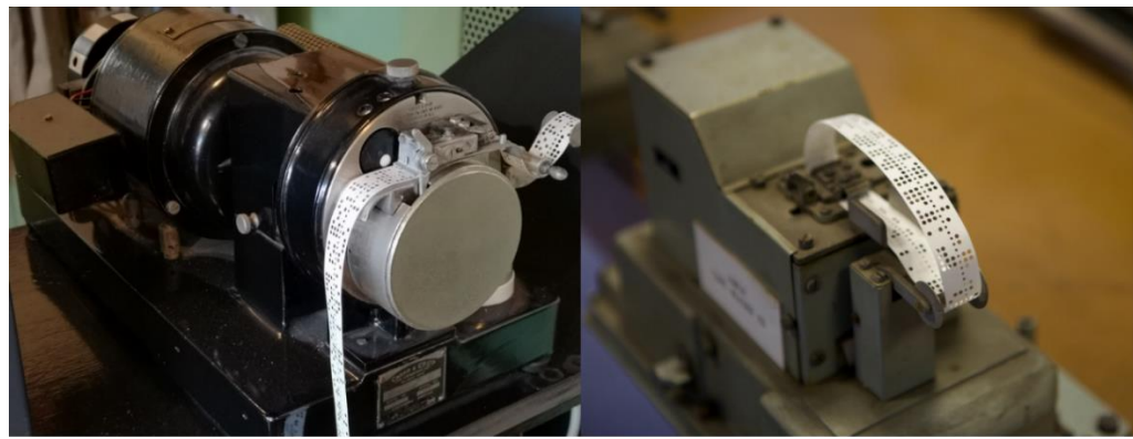
(b) Paper tape reader on the Harwell computer with a small piece of five-hole tape connected in a circle – creating a physical program loop
